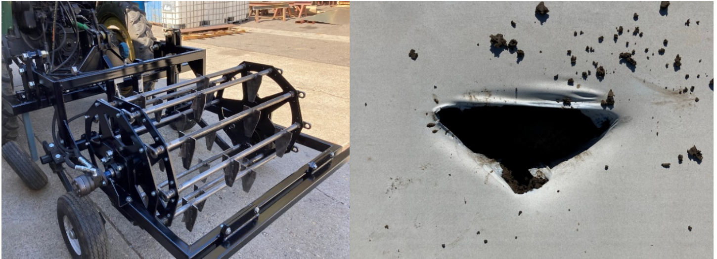
Figure 2. Cross Hole Puncher (left) and example of punched hole (right).
