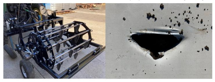
Figure 2. Cross Hole Puncher (left) and example of punched hole (right).
