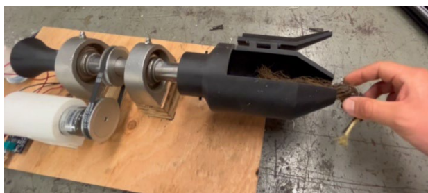
Figure 1. Prototype 1 of a bareroot wrapping mechanism. The tension in the PVA material while wrapping was found to be desirable, however, the loading mechanism was too slow.
