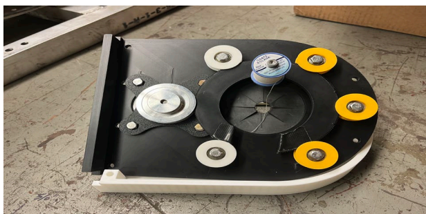
Figure 2. Prototype 2 of a bareroot wrapping mechanism. This design included both loading and manufacturability improvements, however, it lowered the tension consistency as the PVA material was wrapped around bareroots.
