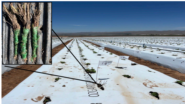
Figure 3. Commercial field testing of a custom PVA/glycerol material. This material retains all beneficial qualities of commercially produced PVA thread, while allowing flexibility and control of components and material characteristics.
