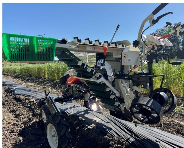
Figure 4. A modified sweet potato transplanter that was used to test planting concepts such as conveyance methods, material handling, and a plant insertion systems.
