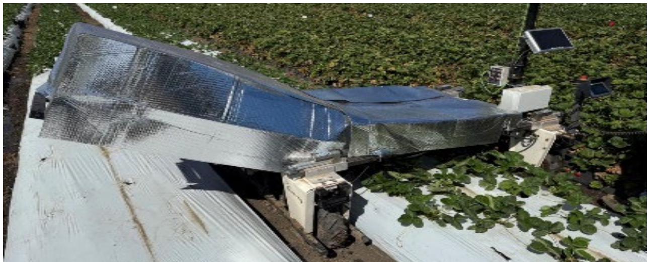
Figure 2. Laser runner cutter mounted on a Farm-NG Amiga during field testing.
