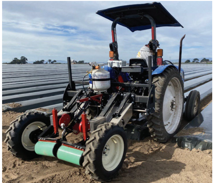
Figure 2. The Heated Hole Puncher operating in Moss Landing, CA.
