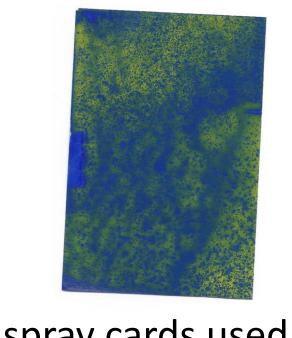
Water sensitive spray cards used to evaluate spray coverage.
