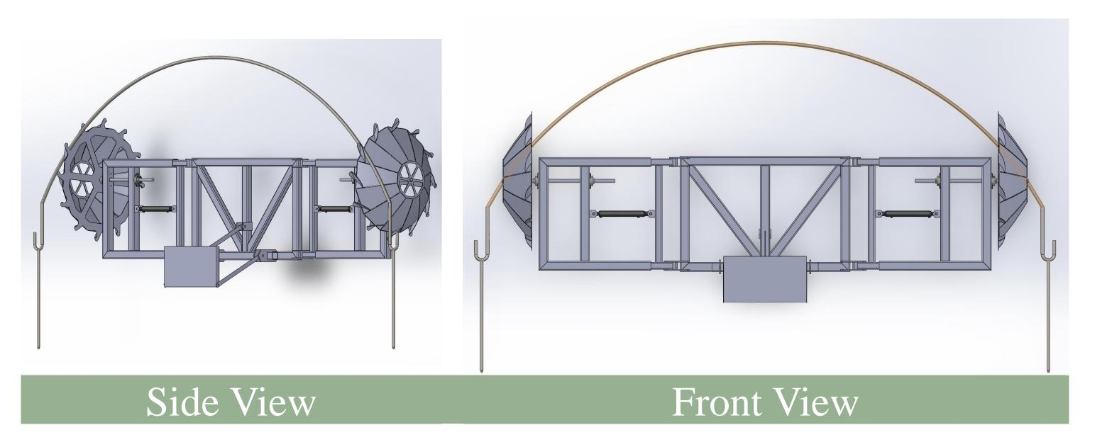
Fabrication process began with the center frame, moved outwards to the extension wings and removal wheels, and finalized with the hydraulic motors, valves, and hose routing.
