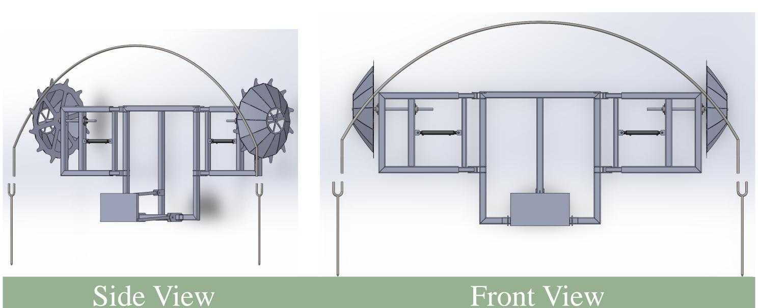
Fabrication modifications began by disassembling the implement, removing the wings, including the hydraulic valves and hose routes, and modifying the center frame.
