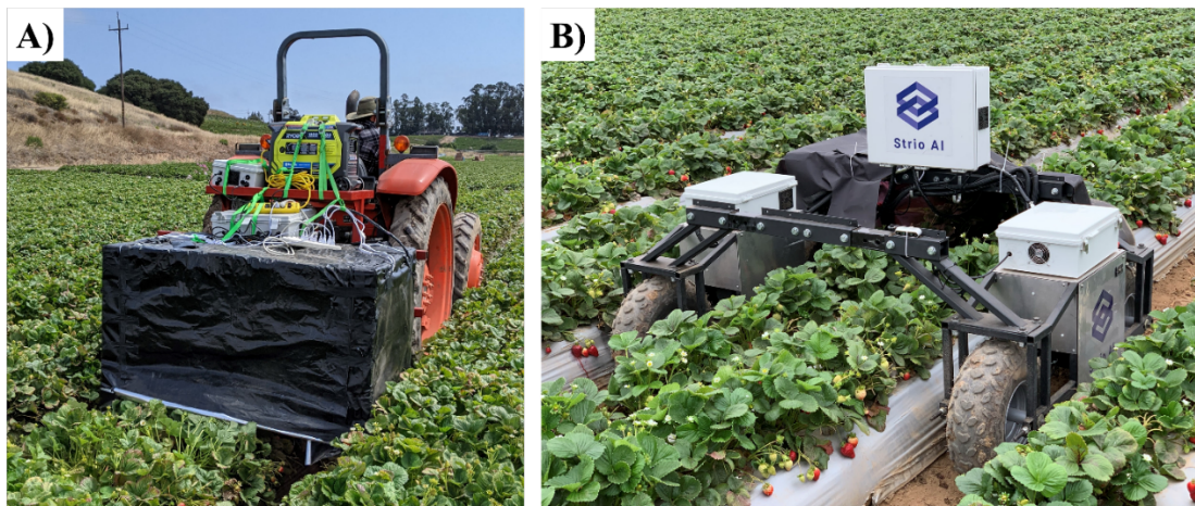
Figure 2. A) Tractor mounted enclosed data collection platform and B) Strio AI robotic platform.
