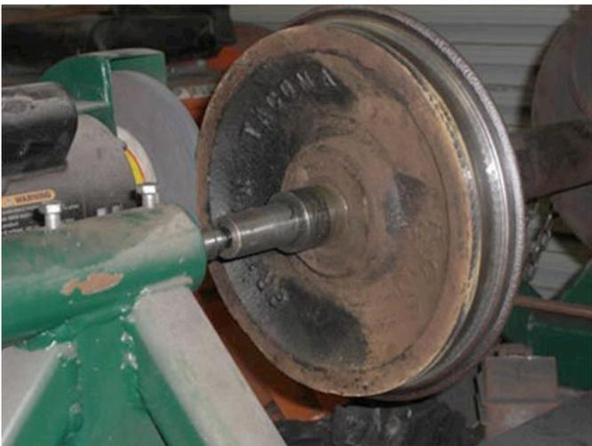
Wheel grinder surfing motor car's wheels
