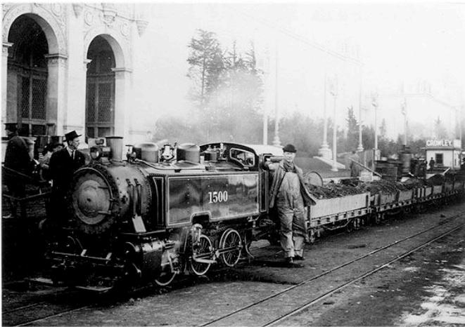
Figure 2. Overfair work train; locomotive No. 1500, type 0-6-0T with five flat cars. SPRS No. 1913-1915 LMM-0018, Al Smith collection
