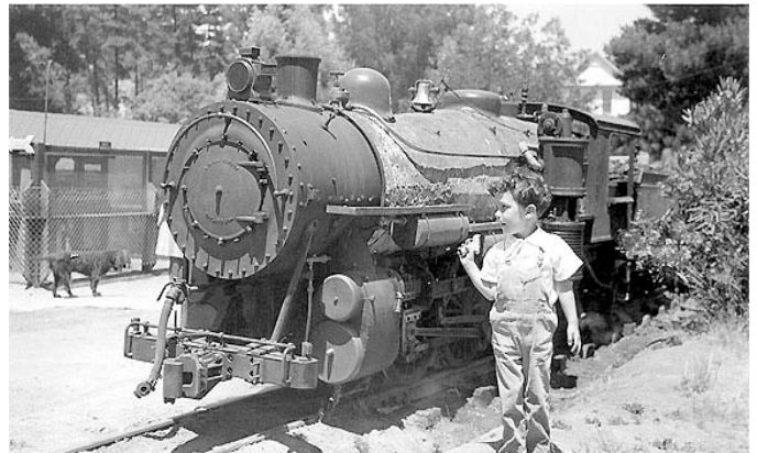
Overfair Railway locomotive 1913 at the Oakland Zoo, 1941-1945. Left side view: Note that this photo shows a partial jacket or covering on the boiler, as evidenced by the shadow of a jagged edge just below the horizontal pipe and above the boy's head. Left background: MacDermot's dog in front of the monkeys' cage.
