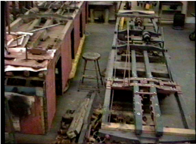
As parts were taken off the original car, they were drawn to scale, & new parts were made or old parts cleaned and painted.
