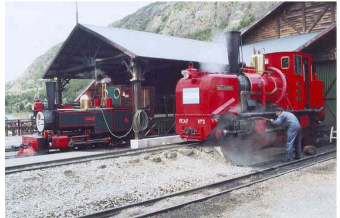
Locomotives of "the Train at the End of the World", the Ferrocarril Austral Fuegino (FCAF). Left, No. 3, 2-6-2T CAMILA; right, No.2, 0-4-0+0-4-0 NORA. Photo from the FCAF website.
