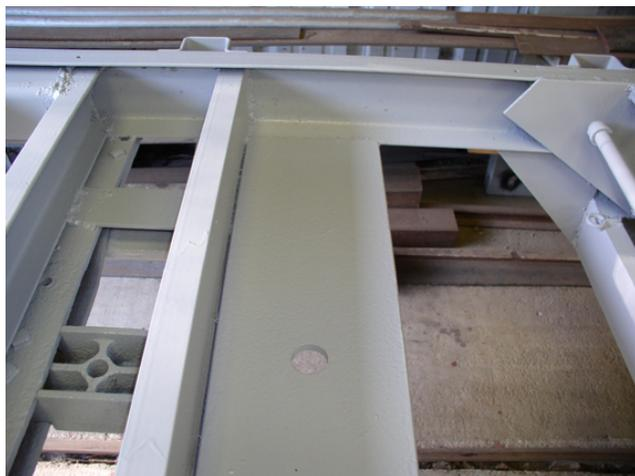
Old and new bolsters in place on the rebuilt car
