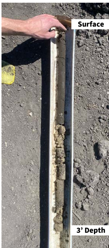
Figure 2. 4' soil core collected using a 4" soil core driven by a gas-powered post pounder
