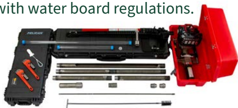
Figure 1. Deep soil corer kit. This one uses a gas-powered post pounder to drive 4" cores to 8'. https://www.ams-samplers.com/gas-powered-core-sampling-kit/
