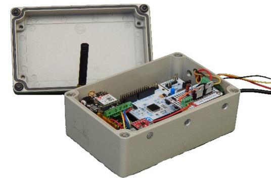
**Figure 1: Windturbine LifeLine prototype**
