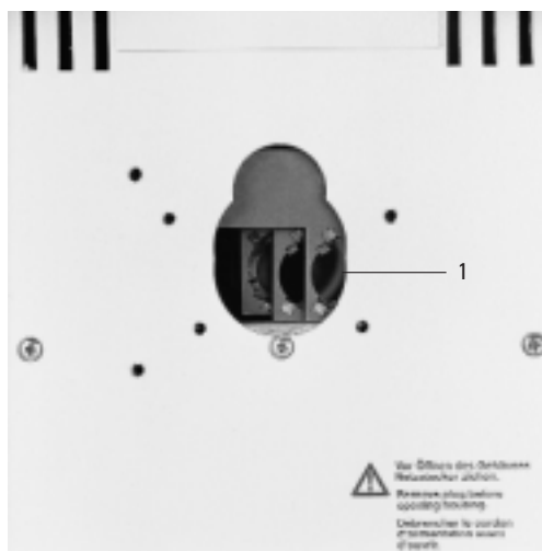
Fig. 73 Back view of microscope without lamphousing mount 1 Filter, 20mm diameter, can only be fitted by service technician
