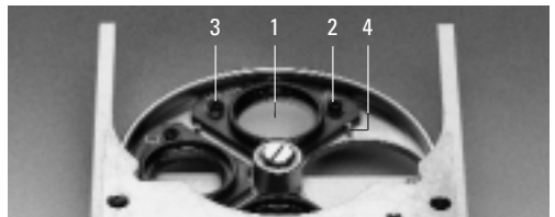
Fig. 35 ICR prism disc 1 ICR objective prism in mount, 2 Code letter (e.g. A), 3 Fixing screw, 4 Stop pin
