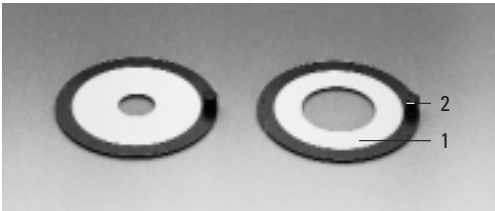
Fig. 18 Round stage inserts 1 Steel ring with inner hole of 20 mm, 30 mm, 40 mm, 2 Grip button, can be screwed off
