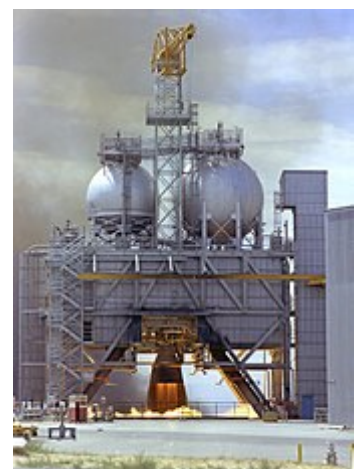
Test firing of an F-1 engine at Edwards Air Force Base
