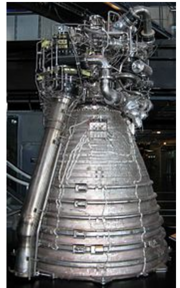
It uses a similar cycle design to the Vulcain engine for the Ariane 5 rocket, with the turbopump exhaust gases piped directly overboard.
