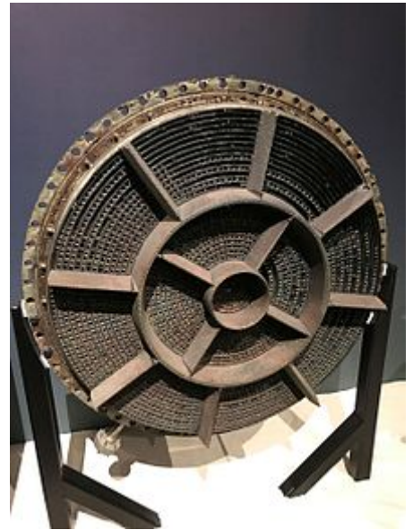
Recovered F-1 engine injector from Apollo 12 mission on display at the Museum of Flight in Seattle.
