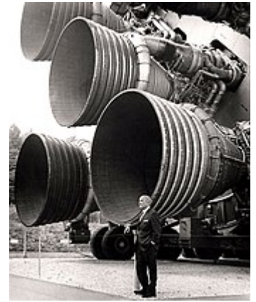
Wernher von Braun with the F-1 engines of the Saturn V first stage at the U.S. Space and Rocket Center
