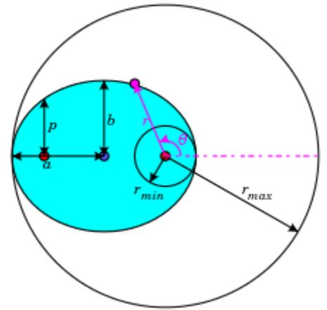
Figure 4: Heliocentric coordinate system  $(r, \theta)$  for ellipse. Also shown are: semi-major axis  $a$ , semi-minor axis  $b$  and semi-latus rectum  $p$ ; center of ellipse and its two foci marked by large dots. For  $\theta = 0^\circ$ ,  $r = r_{\min}$  and for  $\theta = 180^\circ$ ,  $r = r_{\max}$ .
