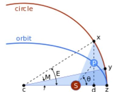
Figure 5: Geometric construction for Kepler's calculation of  $\theta$ . The Sun (located at the focus) is labeled S and the planet P. The auxiliary circle is an aid to calculation. Line  $xd$  is perpendicular to the base and through the planet P. The shaded sectors are arranged to have equal areas by positioning of point y.
