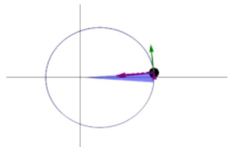
The same (blue) area is swept out in a fixed time period. The green arrow is velocity. The purple arrow directed towards the Sun is the acceleration. The other two purple arrows are acceleration components parallel and perpendicular to the velocity
