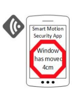
The Smart Motion Sensor utilizes a 1.5V 3000mWh Liion battery, power optimization, and 0.5W small solar panel for self-sustainability so that no maintenance is required during the product lifetime. It uses and accelerometer(BMI160) to detect impacts and window movement. Upon detecting window movement, an optical time of flight sensor(VL53L1X) is woken up to measure window distance.
