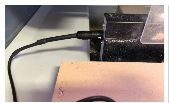
24. Connect the Z-sensor to MDX-50 as shown on the photo.
