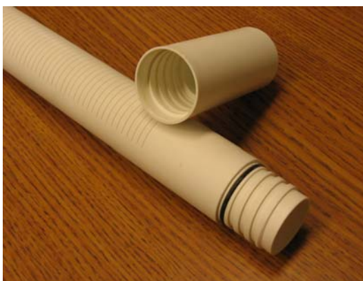
Picture 1: Biofilm sampler with one cap removed. Made by Bob Pease at the Unocal Central Coast Group. The sampler has a 1-inch diameter.
