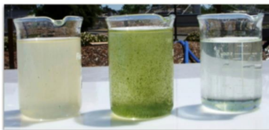
Figure 2. Wastewater treatment and effective bioflocculation of algae at the SLO pilot ponds, June 2012. (Left) Primary clarifier effluents feeds the ponds. (Center) Bioflocculated algae grow and perform treatment. (Right) Settled pond effluent after 30 minutes in a continuous-flow settling tanks.
