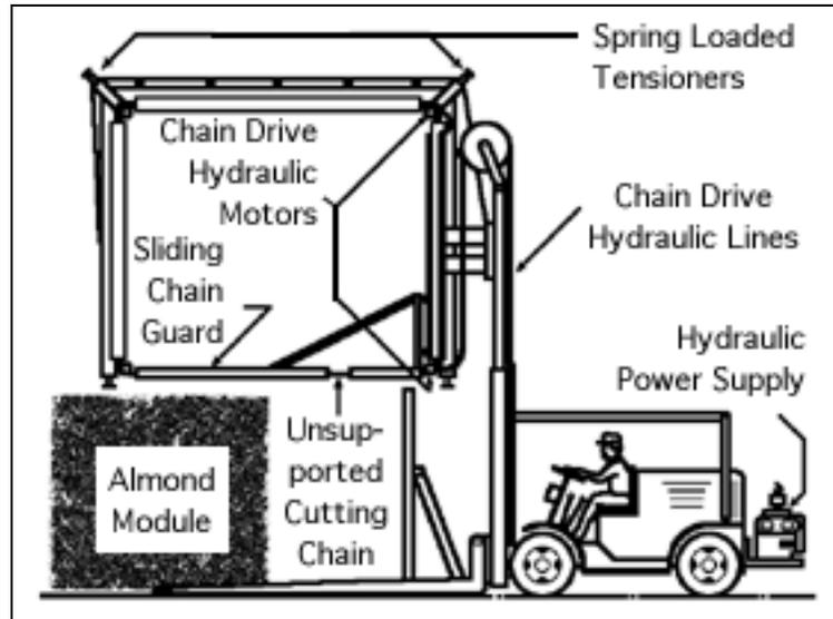
Figure 1. Proposed module cutting machine.
