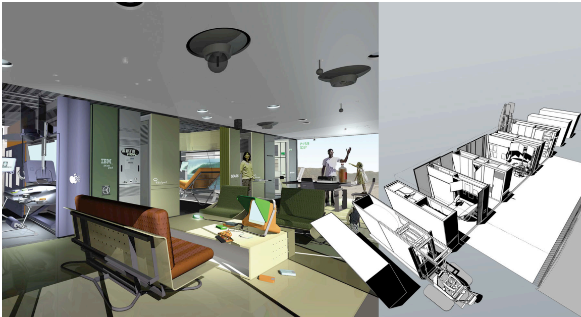
This project features a system of program cabinets that can be slid back and forth within the available volume. The occupants are able to create program-specific spaces between the cabinets as desired, and to eliminate that space and re-dedicate it to another program as interests change simply by repositioning the cabinets. (image: Jones, Partners: Architecture)
