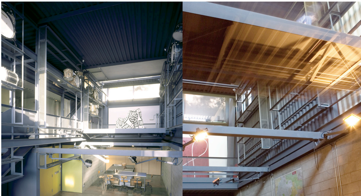
This residence includes a repositionable mezzanine that can be rolled along the length of its main volume, and can be joined with a small street-facing balcony to make a larger indoor/outdoor space. (image: Jones, Partners: Architecture)
