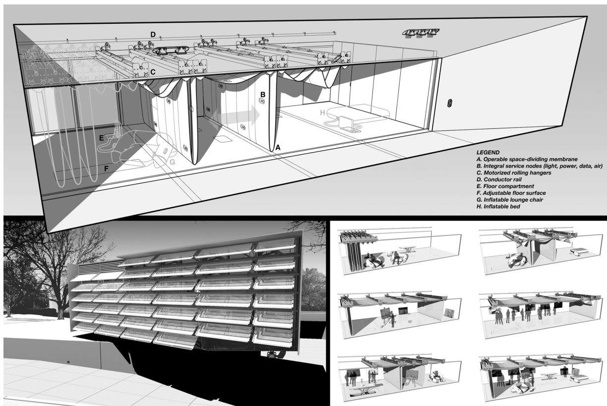
Fig. 2 The DRAPE Artist Residence and Gallery achieves formal multiplicity by means of an operable space-making membrane, which also contains integral power, data, light, and air. In combination with an assortment of inflatable furniture elements, this membrane affords the occupant a high degree of control in how the space is formally redefined with regard to its social, spatial, and programmatic relationships. (image: Doug Jackson)
