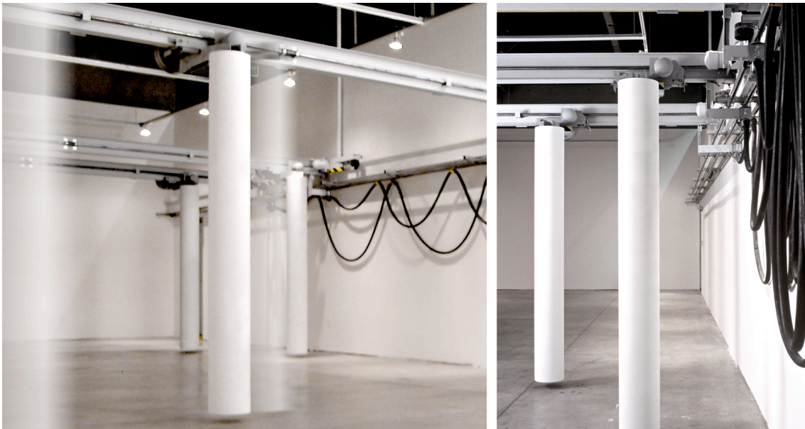
FIGURE 3: Shuffle (Los Angeles, California, USA) by Jones, Partners: Architecture, 2003. This installation at the Southern California Institute of Architecture demonstrates a prototype system for re-configurable architectural space-making elements. In this case, three columns can be repositioned in order to allow individuals to create different architectural relationships within the gallery space. (Image courtesy of Jones, Partners: Architecture).
