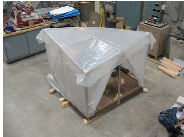
Figure 4: Version 1 built at half-scale using composite materials and plastic sheeting.
