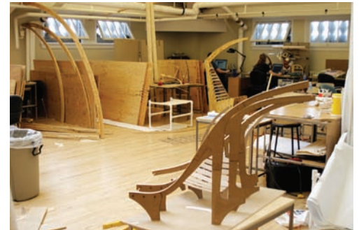
From Scale Model to Full Size: what was easy was done quickly, but testing how materials curve across the vertical elements was avoided. ▼
