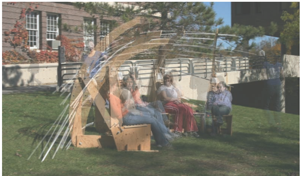
Simple Structure Complex Behavior: after user testing of a preliminary rigid seat mock-up, a flexible spring joint was added which was then connected to a flexible skin. When one user leaned back in their seat, the skin moved affecting others in the circle. ▲
