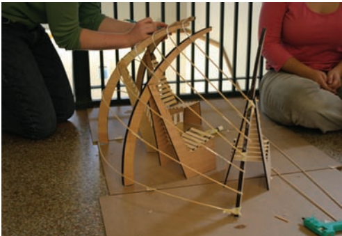
Model as Prototype: model scale based on material thickness. Wood bents measured at scale and then digitally modeled. ▲
