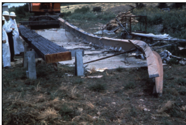
Figure 4: This photo shows a sixteen-inch, 40 lb/ft steel beam (W16x40) and a 7"x 21" glulam beam following fire testing under full load. The steel beam collapsed after only 30 minutes of exposure while the glulam member remained straight and true, charring on \frac{3}{4} " of exposed surfaces.
