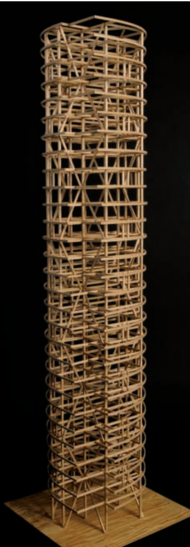
A team of architectural and civil engineering students designed and built a 1/72-scale building from balsa wood (left) for the EERI Seismic Design Competition.
