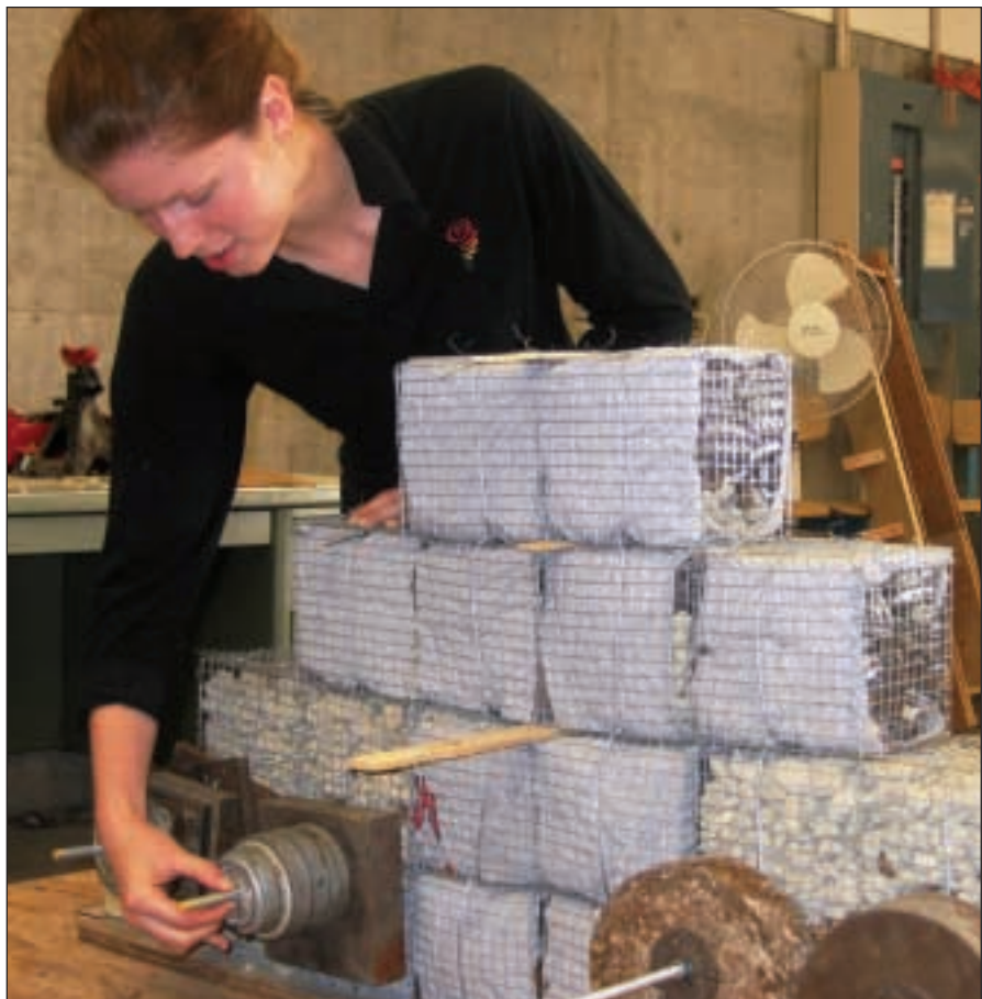
Amy Ransom (above) tests gabion wall samples on the shake table in the Seismic Lab as part of her thesis project to investigate their use for structures in under-developed countries.
